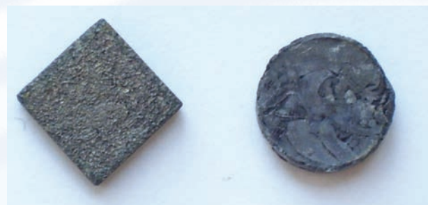
Figure 1. Rhombic tablet of NiZr alloy (left) and round tablet of Zr (right).
