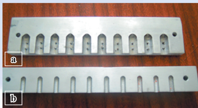
Figure 1. The metallic molds for preparation of suppositories core (above) and outer layer (below). a) metallic mold for outer layer; b) metallic mold for core.
